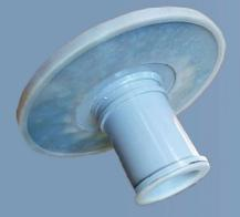
Drain nozzle repair is used to repair small or large damages found on the reactor's floor. The patch is made from CS/SS core and covered with thick PTFE/PFA lining from all sides. It reaches from the reactor's floor down to the sealing face of the drain nozzle. By the external tightening system and the PTFE flexible sealing it is good for working at -1 / barg and temperature cycling. Repair area ranges from 100 mm to 500 mm.
